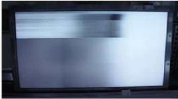
Horizontal Block Gate TAB IC Defect
